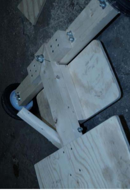
Seat Bottom installed, brake installed, block and foot rest installed. Place foot rest far enough from front axle that steering is not impacted. Adjust brake location as necessary to ensure all scouts can reach while wearing shoulder belt.
