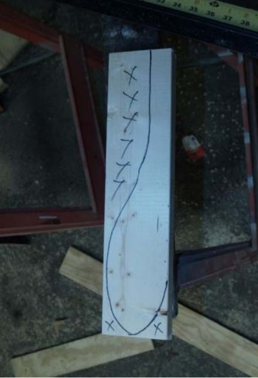
Brake – Shape drawn on block, cut and sand to final shape, wrap with bicycle tire, upside down rubber backed carpet strip, or other material to act as brake pad
