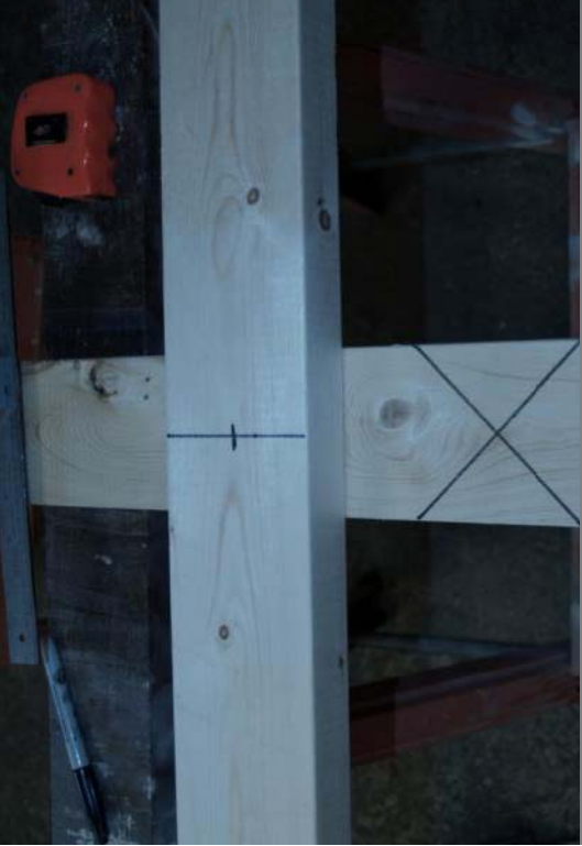
Front Axle -- Centers marked on axle and frame
