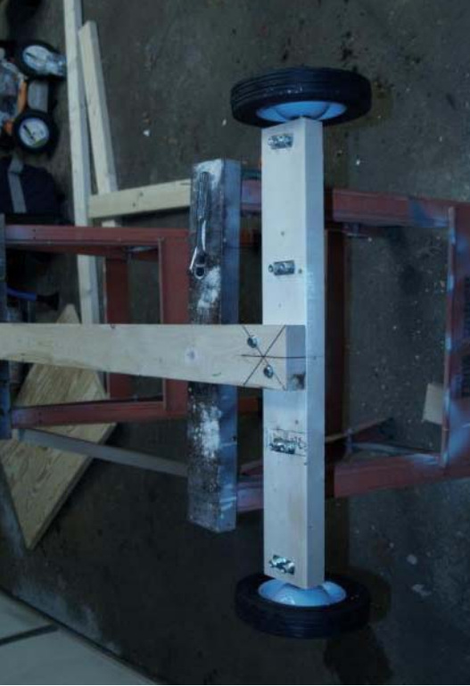
Rear Axle Top – Showing U-Bolts and axle bolted to frame. U-bolt nuts where replaced with Nyloc nuts, supplied nuts screwed on top to cover threads.
