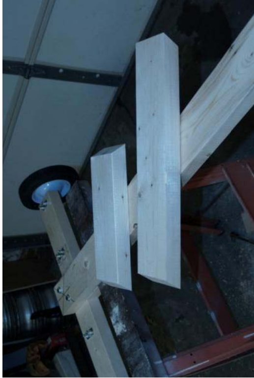
Seat Back – Brace and support pieces have been cut (30 deg angles)
