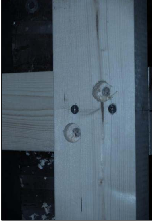
Rear Axle – Bolt holes completed, countersink must be large enough for socket
