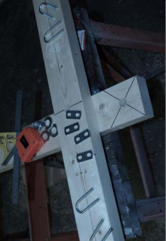
Front Axle -- Holes drilled for center pivot bolt and threaded rod u-bolts
