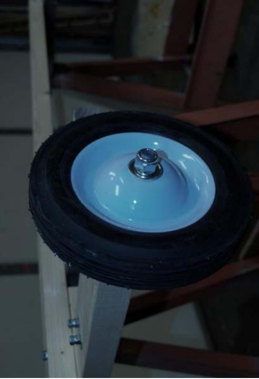
Rear Axle - Shows Wheels fixed with Nyloc nut, two nuts on u-bolts can be seen in background. Axle is 1/2 inch rod.
